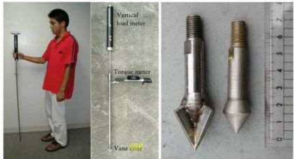
Fig. 166.2 Method of estimating cohesion and friction angle by VCST
